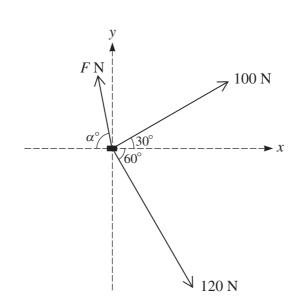
A small box of mass 40 kg is moved along a rough horizontal floor by three men. Two of the men apply horizontal forces of magnitudes 100 N and 120 N, making angles of 30° and 60° respectively with the positive x-direction. The third man applies a horizontal force of magnitude F N making an angle of  $\alpha^{\circ}$  with the negative x-direction (see diagram). The resultant of the three horizontal forces acting on the box is in the positive x-direction and has magnitude 136 N.
